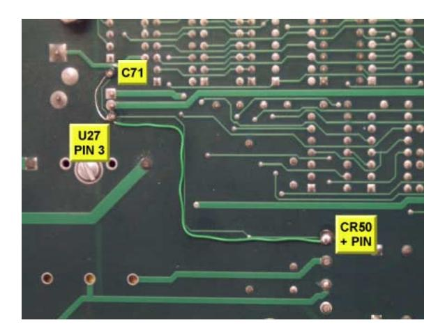
Beginning with HW Rev 1.63 a production change has been made to improve the reliability of the trace.
