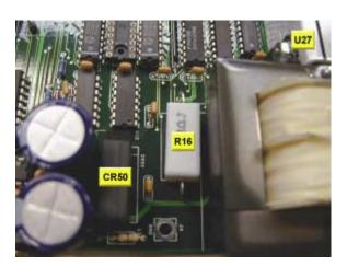
To determine if the loss of Vaa is due to a broken foil trace, simply remove power to the board and measure for continuity between pin 3 of U27 (pin 3 is the pin closest to the power transformer) and the end of R16 closest to the edge of the board. If you do not measure continuity, the trace is broken. If you do measure continuity, the trace is intact and your board will require factory service.
